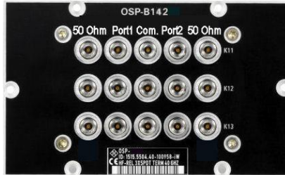
Figure 5-49: Module R&S OSP-B142 (variant .03 with 3 DP3T switches)
